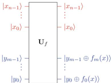
**Fig. 3.8** Quantum gate that evaluates function  $f(x)$ . The function’s domain is loaded into the register  $|x\rangle \equiv |x_{n-1} \dots x_1 x_0\rangle$  shown in red. Following processing by  $\mathbf{U}_f$  register  $|y\rangle \equiv |y_{m-1} \dots y_1 y_0\rangle$  shown in blue, maps into  $|y \oplus f(x)\rangle$ . In that register,  $f(x)$  is evaluated in entries where  $y = 0$
