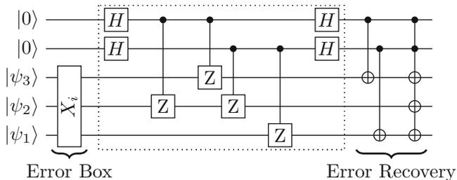
**Fig. 9.3** A three-qubit error correcting code for a single flip error. The gates inside the dotted line constitute the syndrome measurements. The error is generated by phantom gates  $\mathbf{X}_1 = \mathbb{1} \otimes \mathbb{1} \otimes \mathbf{X}, \mathbf{X}_2 = \mathbb{1} \otimes \mathbf{X} \otimes \mathbb{1},$  or  $\mathbf{X}_3 = \mathbf{X} \otimes \mathbb{1} \otimes \mathbb{1}.$  The error recovery segment includes a sequence of Toffoli gates discussed in Mathematica Notebook 9.2
