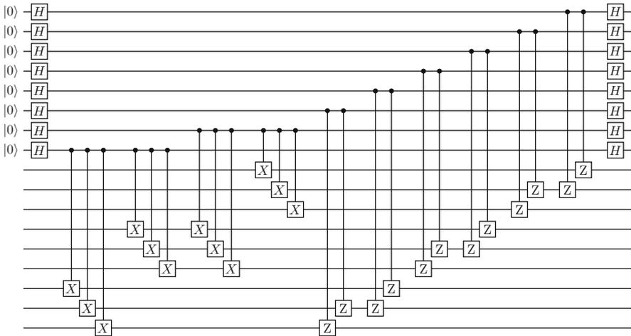
**Fig. 9.8** Syndrome circuit for Shor nine-qubit code. The code words  $|0\rangle_{9L}, |1\rangle_{9L}$  are subjected to an error box consisting of all possible single-qubit errors. The nine-qubits are represented by the first 9-wires (starting from the bottom of the figure), and the eight ancillary qubits by the last 8 wires
