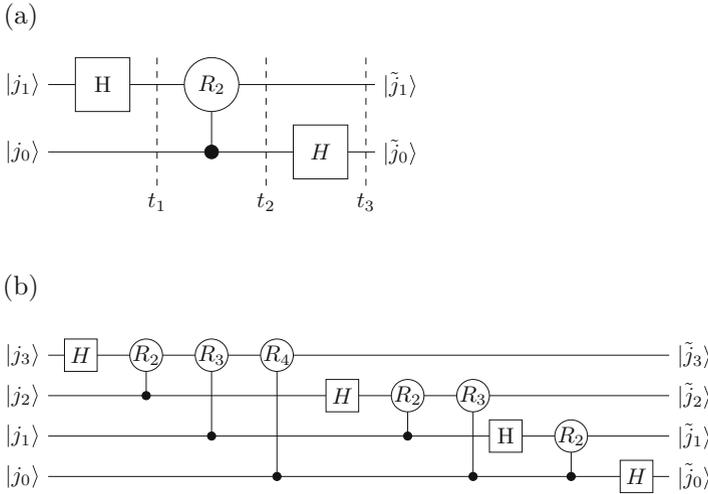
**Fig. 4.2** Panel (a): A two-qubit circuit for operator **QFT**. Panel (b): four-qubit circuit.  $|\tilde{j}_0\rangle = |0\rangle + \exp(2\pi i [.j_0]) |1\rangle$ ,  $|\tilde{j}_1\rangle = |0\rangle + \exp(2\pi i [.j_1 j_0]) |1\rangle$ , etc. States **QFT**  $|j_{n-1} \dots j_1 j_0\rangle$  are recovered by the action of a qubit swap operation on  $|\tilde{j}_{n-1} \dots \tilde{j}_1 \tilde{j}_0\rangle$
