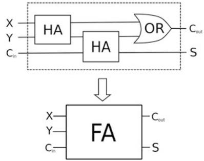
**Fig. 3.4** An adding circuit, for a pair of two-bit registers
