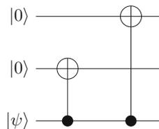
**Fig. 9.2** Syndrome and error recovery for a flip error in the first qubit of the codeword
